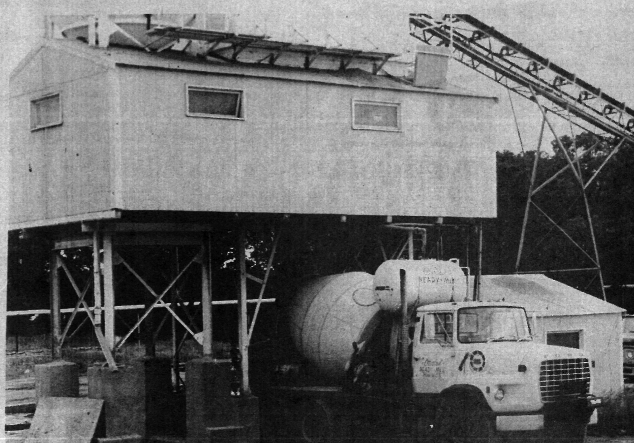
READY MIX —This Ready Mix truck awaits a load from the mixing plant. The cement was to be delivered to a job site in the area. (Marilyn Johnson photo)
